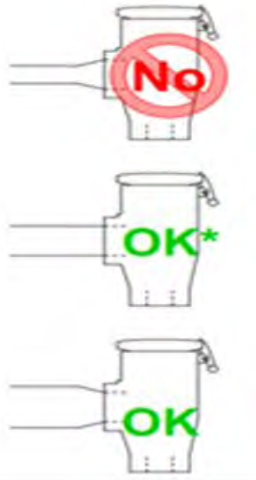
Figure 2: Outlet Piping Requirements
