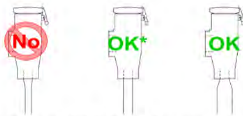
Figure 1: Inlet Piping Requirements
