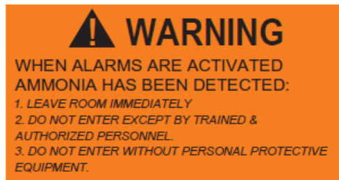
Figure 2: An Illustration of the Alarm Signage with the Audio/Visual System
