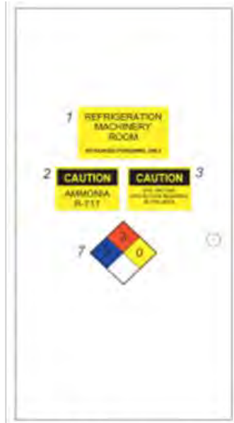
Figure 1: Machinery Room Door Required Signage
